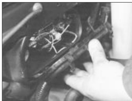
5.1 Removing the cover from the rear of the headlight
