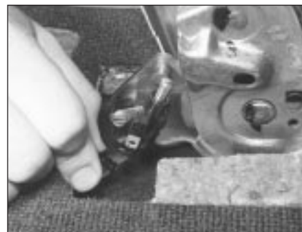
4.44 Disconnecting the multi-plug from the handbrake lever
