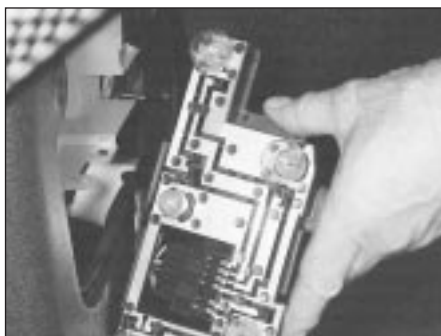
5.27C Removing the rear light cluster (Saloon)
