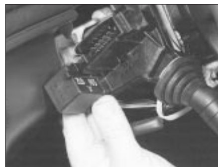
4.23 Removing the direction indicator, dipped beam and hazard flasher multi-function switch. Direction indicator relay (flasher unit) is attached
