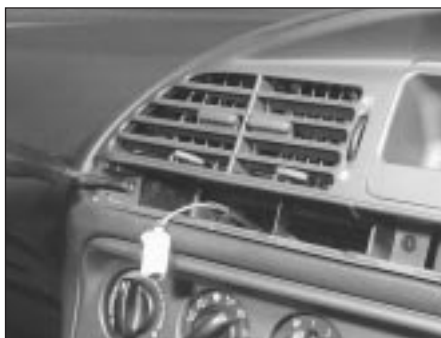
10.8B . . . and the remaining screws . . .
