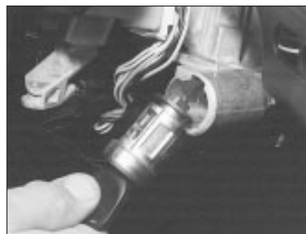
4.3B . . . and withdraw the ignition lock barrel
