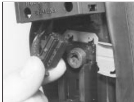
20.3A Disconnecting a movement sensor multi-plug
