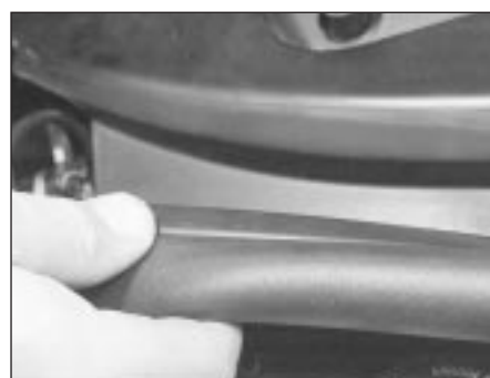
16.5 Removing the bonnet sealing strip
