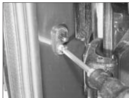
4.57A Unscrew the cross-head screw . . .
