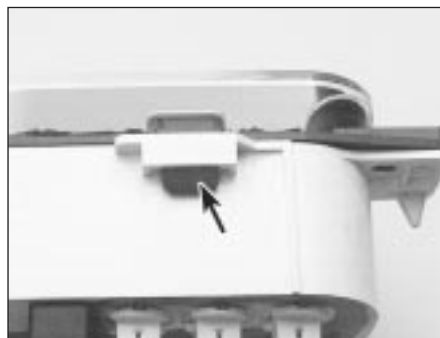
11.2 Bezel retaining lug on the instrument panel
