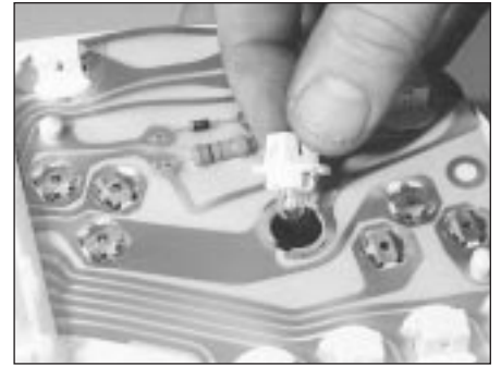
6.11 Removing a bulb from the rear of the instrument panel
