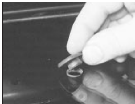
22.12B . . . and prise out the rubber grommet
