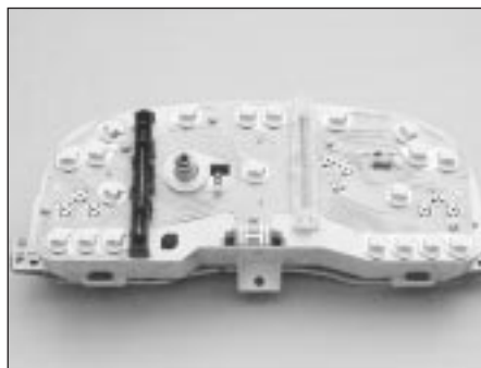
11.1 Rear view of the instrument panel, showing bulbholders
