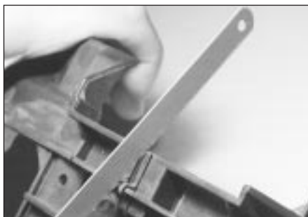
7.8D Using a hacksaw to cut through the middle of the headlight back-piece, in order to fit a new unit
