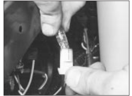
5.10 Pulling the wedge-type bulb from the bulbholder
