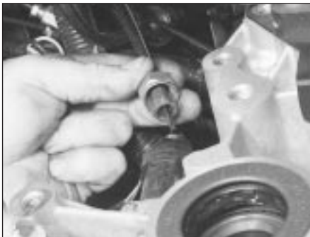
12.9B . . . and disconnect the speedometer cable from the vehicle speed sensor
