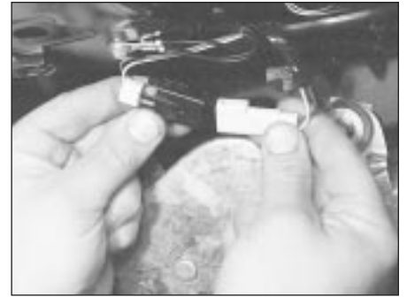
17.4 Disconnecting the tailgate wiper motor multi-plug
