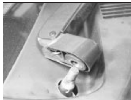
15.5 Removing the wiper arm from the spindle
