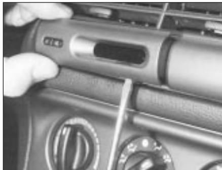
13.2 Prising the clock out of the facia
