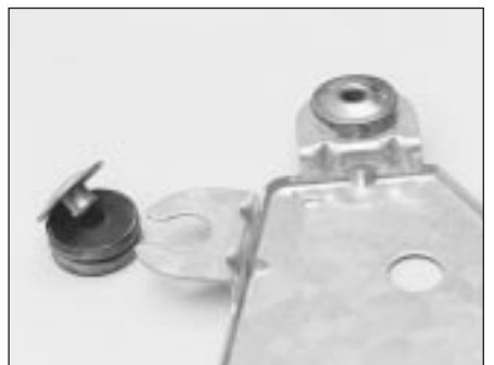
17.7B A mounting rubber removed from the mounting plate
