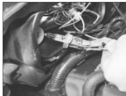
5.5 Removing the headlight (main beam) bulbholder
