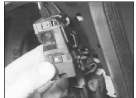
20.3B Removing a movement sensor
