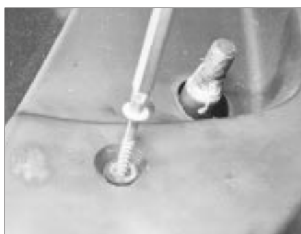
16.3B . . . and remove the upper retaining screws
