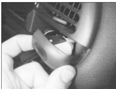
10.6 Removing the foglight warning indicator
