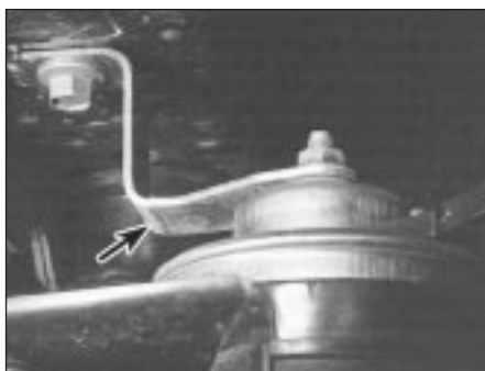
14.4 Horn and mounting bracket (arrowed)
