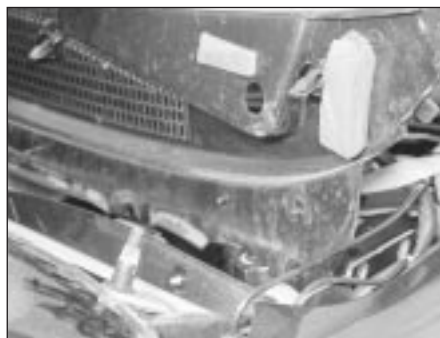
16.6B . . . and remove the grille panel from in front of the windscreen
