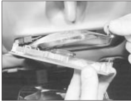
6.5 Lifting the reflector from the interior light
