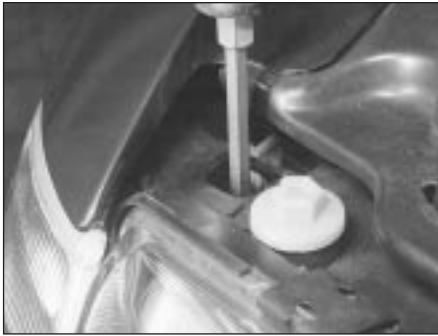
7.10 Loosen the front direction indicator retaining screw
