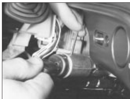
4.3A Depress the locking plunger . . .
