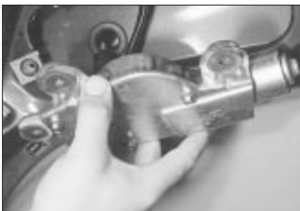
17.6B ... and remove the tailgate wiper motor assembly (Hatchback shown - Estate similar)
