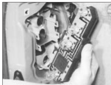
5.27B Removing the rear light cluster (Estate)
