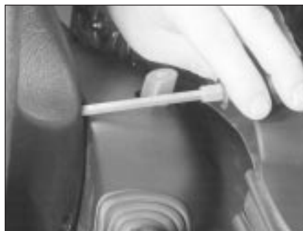
28.3 Unscrewing an air bag mounting bolt
