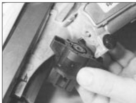
4.4B . . . and remove the ignition switch
