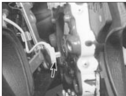
28.4 Disconnecting the air bag wiring multi-plug (arrowed)
