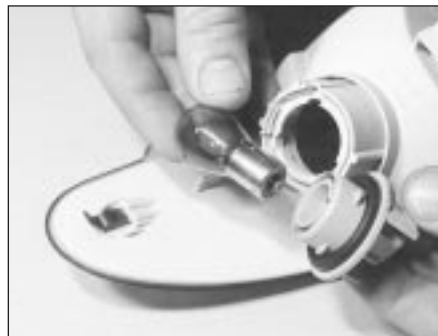
5.15 Removing the front direction indicator bulb
