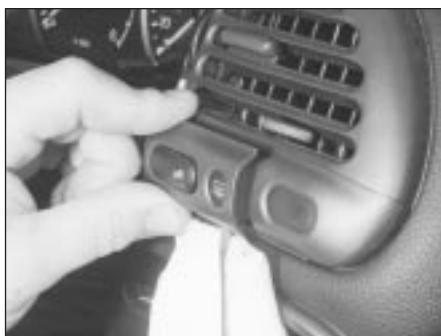
4.49 Prising out the heated rear window switch
