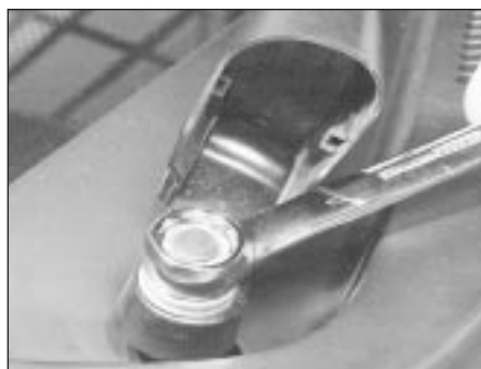
15.3 Loosening the wiper arm retaining nut
