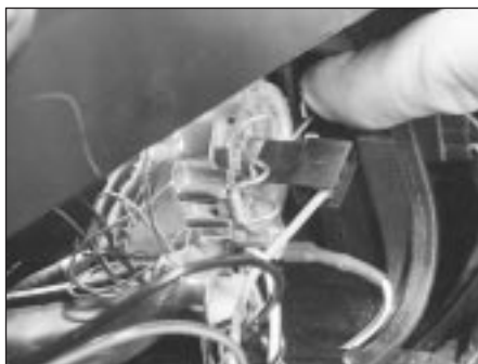
5.2A Release the spring clip . . .
