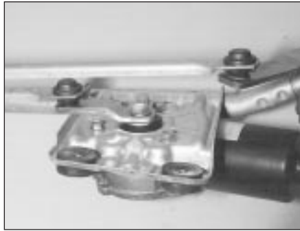
16.10 Wiper motor arm and mounting plate located on the motor
